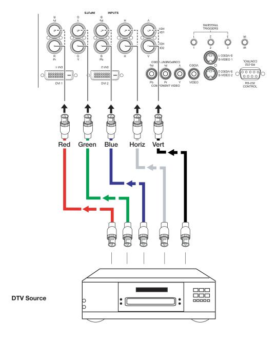
Figure 3-8. Digital (DTV) RGB Connections
