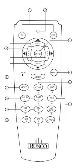
Figure 2-3. VX-2i Remote Control Functions
