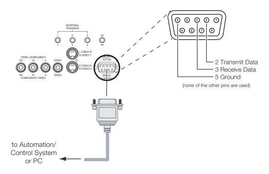
Figure 3-11. RS-232 Control System Connection
