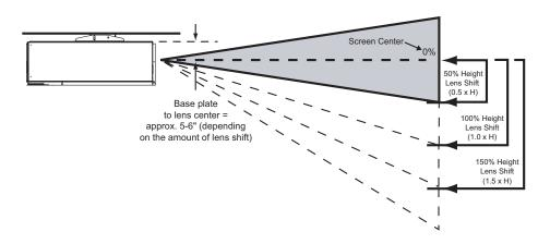
**Note:** This is a general example of lens shift. Lenses vary in their shift capabilities. No particular lens is used in this example.
