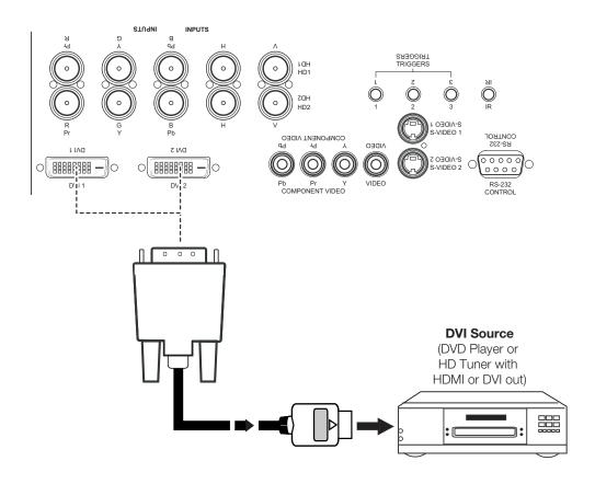
Figure 3-7. DVI Source Connections
