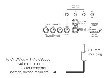
Figure 3-12. Connecting 12-Volt Trigger Outputs
