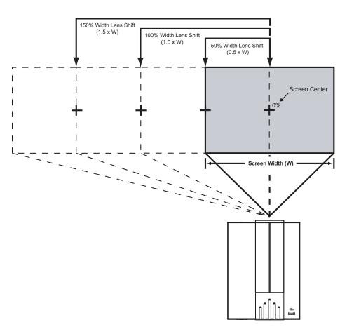
**Note:** This is a general example of lens shift. Lenses vary in their shift capabilities. No particular lens is used in this example.
