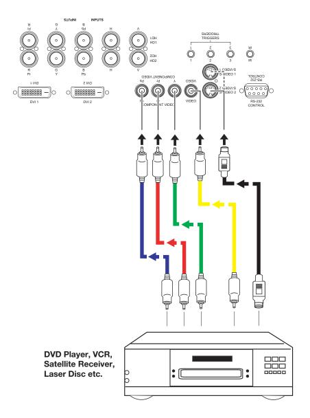
Figure 3-10. Composite, S-Video and Component Video Connections
